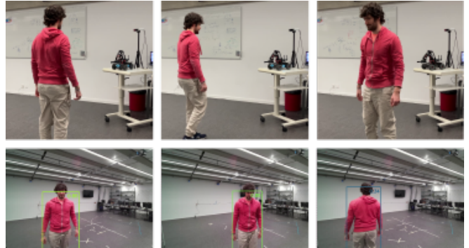
Fig. 1. In a human-robot interaction context, when properly approaching the robot, a user is classified as intending to interact (first two snapshots); otherwise it is classified as non-interacting (right).
