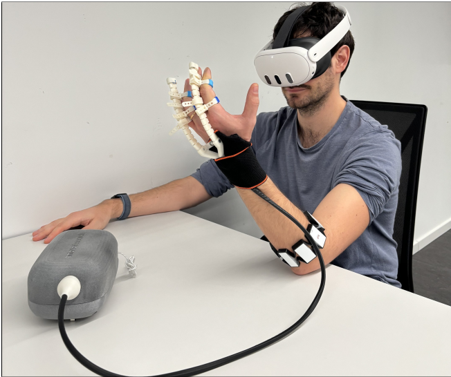
Fig. 2. Enhanced configuration of our setup: an EMG sensor can augment the tool perception skill and open it to interesting rehabilitation applications.
