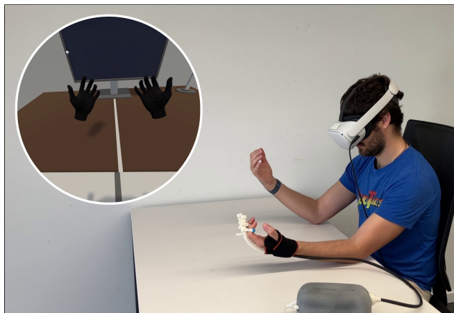
Fig. 1. Our rehabilitation tool for MT. The user wears the exoskeleton at the left hand and the VR headset. In the VR scene, shown in the white circle, the right hand is tracked and rendered, while the left hand is visually mirrored from the right one. The exoskeleton is actuated to move the left hand and match the posture of the right hand.
